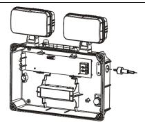
Drill the cable entry point on the side wall. Ensure the provided cable gland is fitted, to maintain the IP65 rating.
