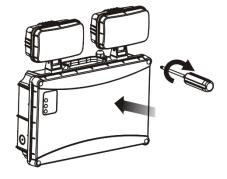
Refit the cover to the body, and secure in place using the four screws.
