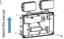
Drill out the four fixing points on the back face. Ensure the fixings are adequately sealed in order to maintain the IP65 rating. Secure the luminaire with four screws.
