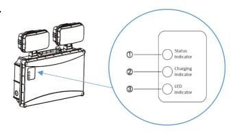
Once the power supply has been reconnected, the green LED indicators on the front of the luminaire should now be illuminated. These green indicators show the battery is charging and there are no faults.
