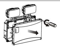
Remove the front cover by loosening the four screws.
