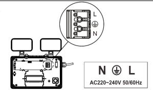
Pass the cable through the cable gland, and wire directly into the terminal block. Secure the mains cable using the internal cable clamp and connect the battery.
