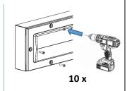
Rest the frame on top of the housing. Insert all M5 screws before fully tightening to ensure alignment.
