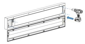
Drill suitable fixings to suit required installation. Please note, it is the contractor's responsibility to ensure the holes are suitably sealed. Failure to do so will invalidate the luminaire's IP rating.
