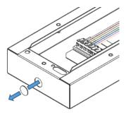
Knockout the semi-shear from the housing if bringing the cable in through the side.
