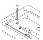
(1) Slide one end of the gear tray into the housing. (2) Then lower the gear tray into place. Secure the tray with the screw that was removed earlier in step 2.
