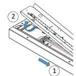
Remove the screw holding the gear tray in place. (1) Push the tray to one side. (2) Lift and tilt the gear tray to remove.
