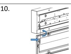
Offer the frame up to the housing. Ensure screw boss on diffuse will align with clearance hole in housing
