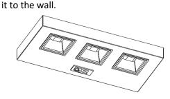
2. Firstly unscrew the 3 screws along the back edge of the fitting. This will release the wall mount bracket.
