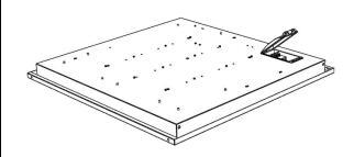
Fitting is supplied as one-piece unit. 595X595mm to rest on 15/24mm exposed T bar
