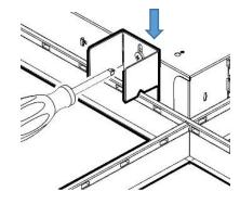
.. each bracket should be adjusted, ensuring fixture is tight against grid / level with tiles where applicable)... exposed T grid shown. Tighten screws on all brackets
