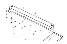
Fit adapter rails to rear of housing using 2No M4x5 self-tap screws as shown
