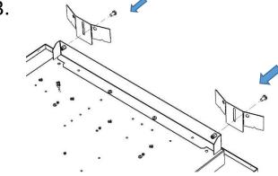
Fit brackets (part bent as shown) to rail – 2 brackets fit one rail - x2
