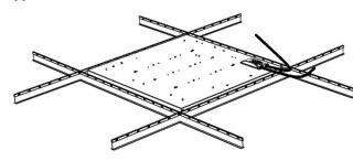
Fitting installed (shown here with loop-in / loop-out cables)
