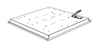
Fitting is supplied as one-piece unit. x2 rails and x4 brackets supplied loose. Fitting measures 599X599mm designed to pull-up <clamp> to various ceilings
