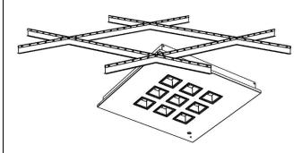
Carefully lift and tilt the luminaire into the ceiling aperture. Fitting will self-locate on grid
