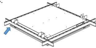
Regardless of ceiling type, the fixture should be offered up in aperture, then all brackets bent as shown – fixture will hang below ceiling....
