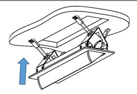
Lift up the springs and raise fitting into the cut out. Use a pattress in the ceiling if required.
