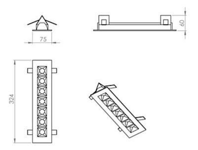
Ceiling thickness 4-25mm Ceiling cut out : 55x304mm
