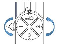
Rotate to select the desired circuit.
