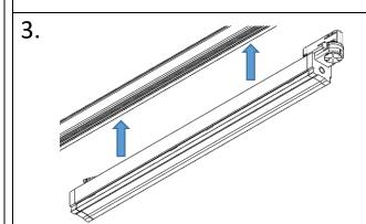
Offer the luminaire up to the track. Ensure both the track adaptor and quarter turn are pushed inside the
