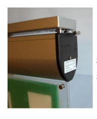
HBE LED M3 suspended Exit signs are available with a selection of ceiling and wall mounting plates. The selected mounting plate should be fitted to the mounting surface using fixings appropriate to the application. Supply cables should be installed according to National Wiring Regulations and should suit the type of mounting arrangement chosen.
