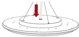
Feed suitable mains cable through grommet in rear of housing.
