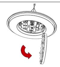
Allow central cover to hang on tether to access the terminal connectors.
