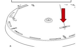
Locate the 4no. suspension holes in the rear of the housing and feed the toggles through the holes provided.
