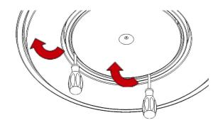
Gently pull the screwdrivers towards the outside of the fitting to release the internal clips. 4.
