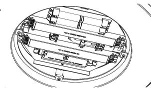
Wire mains cable into the respective terminals. All terminals are labelled for convenience. Ensure cable is clamped using the cable clamp provided.
