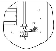
Connect incoming power cable as per diagram on leaflet and use the strain relief provided.
