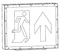
Locate legend in-between the frame and housing when replacing the frame. Fasten frame in place with original screws.
