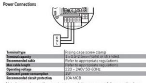
Note: In accordance with current wiring regulations a means of disconnection (e.g. switch) must be incorporated into the fixed wiring.
