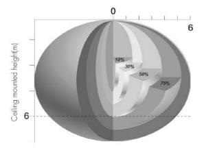
Ceiling mounted detection pattern (m)
