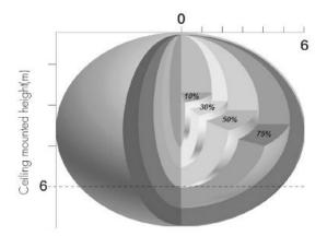
Ceiling mounted detection pattern (m)
