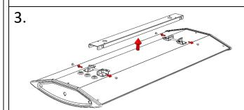
Remove 4x M5 PanPozi screws to release the mounting spine form rear of fitting. Do not remove M6 bolts.
