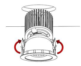
Load spring clips and raise fitting into ceiling aperture
