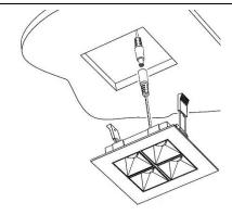
After passing remote gear pack through cutout, connect leads as shown... retract springs fully and offer fixture in to ceiling aperture
