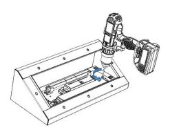
Undo x2 screws and remove the gear tray.
