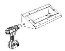
Drill 20mm cable hole in desired location. (Contractor to supply suitable grommet).
