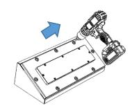
Undo the 8 x M5 6 Lobe Pin Drive screws and remove the frame.
