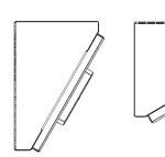
This luminaire can be mounted at either a 60 or 30 degree angle.
