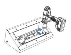
Re secure the gear tray to the body.
