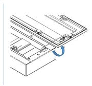
Unpack the luminaire and undo the 10 x M5 6 Lobe Pin Drive screws securing the frame. Remove the frame and proceed to hang it on the tethers.
