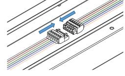
Connect the tray to the housing using the internal loom.
