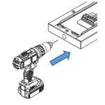
Cornice and slim only - Drill 20mm cable hole in desired location. Drill the rear of the housing if a central cable entry is required instead.
