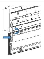
Offer the frame up to the housing. Ensure screw boss on diffuse will align with clearance hole in housing
