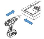
**Slim version only** - Drill alternate cable entry hole position if chosen grommet depth will clash with nutsert.
