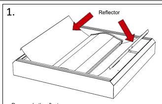
Remove both reflectors. Ensure gloves are worn to prevent the reflectors being marked.
