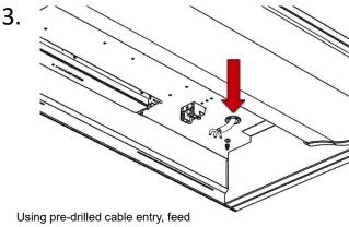
mains cable into the rear of the fitting and wire into relevant terminals.
