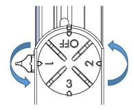
Rotate to select the desired circuit.
