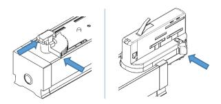
Ensure the quarter turn is aligned correctly and located on the same side as the locking pin for the track adaptor.
