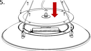
Feed mains cable through the gland and wire into respective terminal block. Ensure cable clamp is used and tighten gland around cable when finished. Replace cover and screws when finished.
