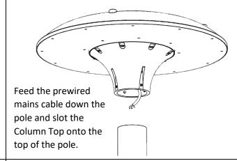
3. Tighten all grub screws using a 4mm Allen key to 11Nm.
