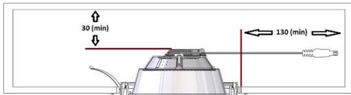
**Emergency Fitting – due to emergency gear box**
