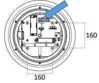
Bring power supply through central grommet and connect it to the terminal block. Then secure the housing to the wall using the 4 fixing points on the back side of the fitting.
