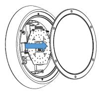
Remove the retaining ring and front diffuser to gain access to the terminal block.
