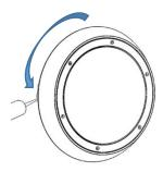
Run Anti-Pick Mastic around the profile of luminaire to ensure the fitting is secure. Must be installed with **anti pick mastic** to meet ligature resistant requirements.
