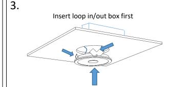
Flex plastic wings into cut-out the push luminaire up until luminaire is secure
