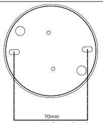
Fixings available for surface fixing.
