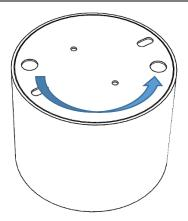
To access ceiling rose, rotate top disc anticlockwise. 3.
