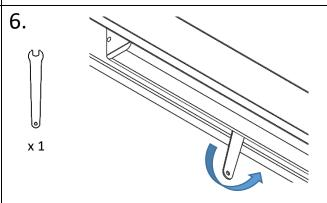
Use the spanner provided to tighten the screws.
