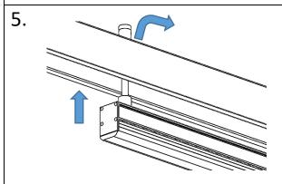
Offer the luminaire up to the brackets, feeding the cables through as you go.
