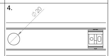
Drill a 20mm hole to each side of the brackets to allow for cable entry.
