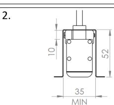
The trough/cladding must be a minimum of **35mm** in width for installation.
