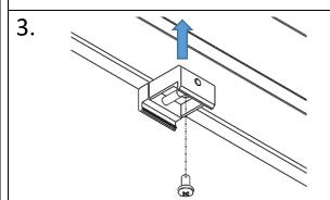
Ensure the clamps are loose and not fully tightened. Proceed to screw them to the desired mounting surface.
