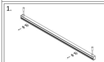
Each fitting will be supplied with 2 mounting brackets and 2 screws.
