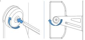
To adjust the angle of the bracket, use an Allen key to loosen the hex bolts on the sides. Retighten these bolts once at the desired angle.
