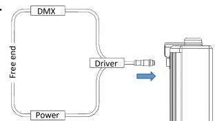
Connect the first fitting to the driver. Then establish a connection with the free end of the cable.
