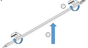
Raise the AluLED module up and 'snap' into place
