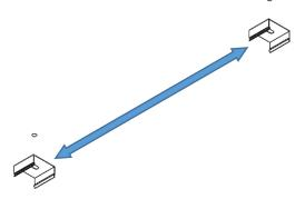
Position the clips in the desired location. The space left between the mounting clips must ensure the module neither bends nor bows.
