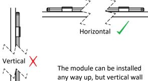
The module can be installed any way up, but vertical wal mounting could lead to the module slipping out of the clips.
