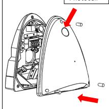
Ensuring all holes drill have been sealed to IP65, refit cover and fasten the screws. Fit cover caps in each hole in the orientation if the keys.
