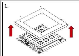
Remove screws and release frame from fitting.
