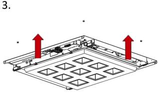
Lift fitting up onto the 4no. Screws. Four keyhole slots in the rear of the fitting should align with the screws.
