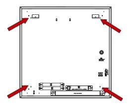
Secure the housing to ceiling using the four screw holes in each corner. (Screw not supplied)
