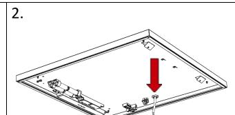
Feed mains cable through the cable grommet and wire into respective terminals. Ensure cable restraint is used.
