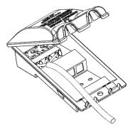
Electrical connection is made via integrated connection back-flap – allows for LEN L1 (emergency) and D1/D2 <or +/- for 1-10v> where specified.
