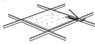
Fitting installed (shown here with loop-in / loop-out cables)
