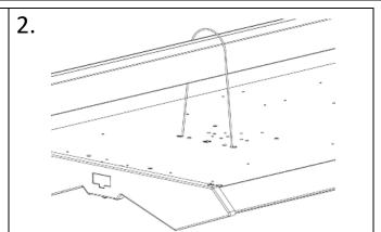
NOTE: THESE TETHERS ARE NOT TO BE THE SOLE METHOD OF INSTALLATION. ONLY TO BE USED AS A PRECAUTION.
