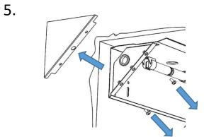
Where fittings are fitted continuously, blanking end covers must be removed (leave in place for start and end of runs)
