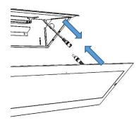
When offering up front LED cover, make sure cable is connected between the two sections! Ensure earth lead is also connected to frame!
