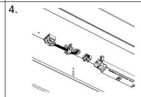
Electrical feed can come through central hole (shown) or through the end plate.
