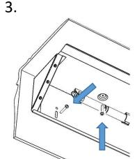
Main housing can be mounted to wall and / or ceiling. It is recommended that it is secured to both.
