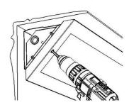
Front LED cover is secured to main housing via the M4 screw at each end – tighten sufficient to ensure contact with both wall and ceiling – do not over-tighten. Fit 10mm white plugs to complete installation
