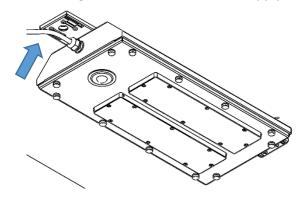
4. Ensure any excess cabling is neatly stored behind the ceiling.
