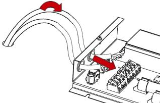
4. Close attention should be payed to the labelling of the cables. Flex 1 and Flex 2 cables should be connected to respective terminal blocks.
