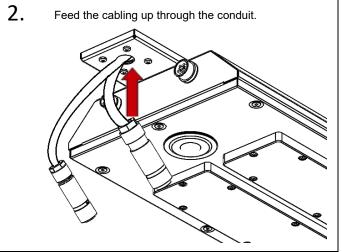
Connect the luminaire head cabling to the remote gear box. Ensure cable restraint is used.
