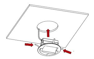
5. The springs will pull the fitting up flush with the front face of the ceiling tile.
