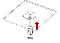
Feed the Driver and 3 pole connector through the cut out into the ceiling void above.
