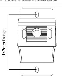
Remove two screws from the cover and keep safe. Open the cover to reveal the cable entry and column top mounting points.
