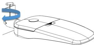
Using the 4mm Allen Key, tighten all the grub screws slightly so the fitting can still rotate.
