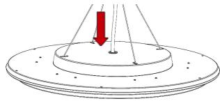
Feed suitable mains cable through grommet in rear of housing.
