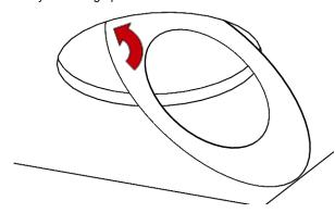
4. Install the downlight into the oval infill ring as if you were installing directly into the ceiling. Refer to the Product specific
