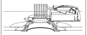
The downlight will need to be centralised in the ceiling aperture to ensure no gaps are visible.
